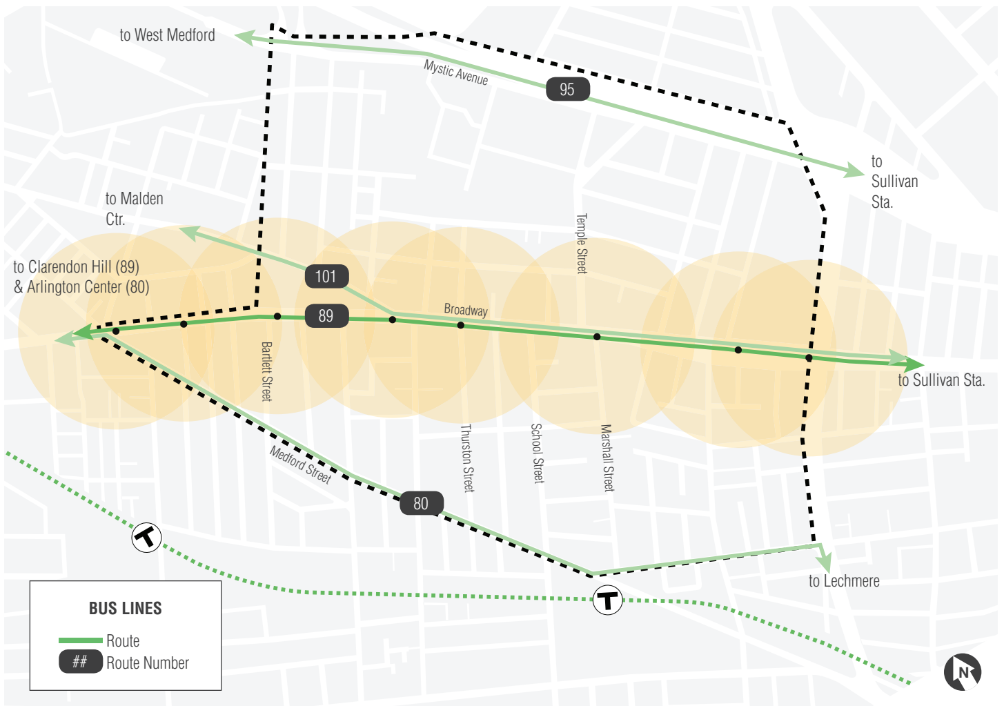
Below: The 89 bus route with 1/8 mile walksheds shown. Where walksheds overlap, service might be redundant.
