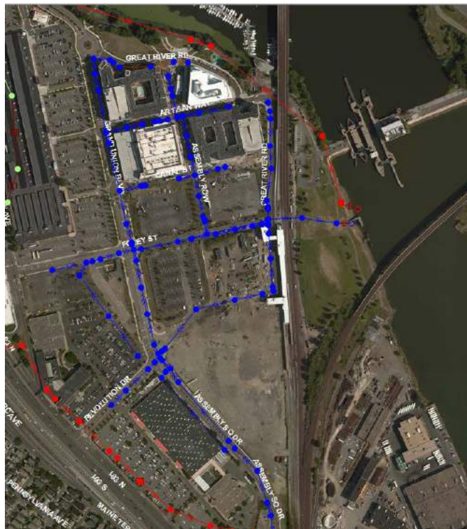
Figure 2. Assembly Square model general pipe layout view
