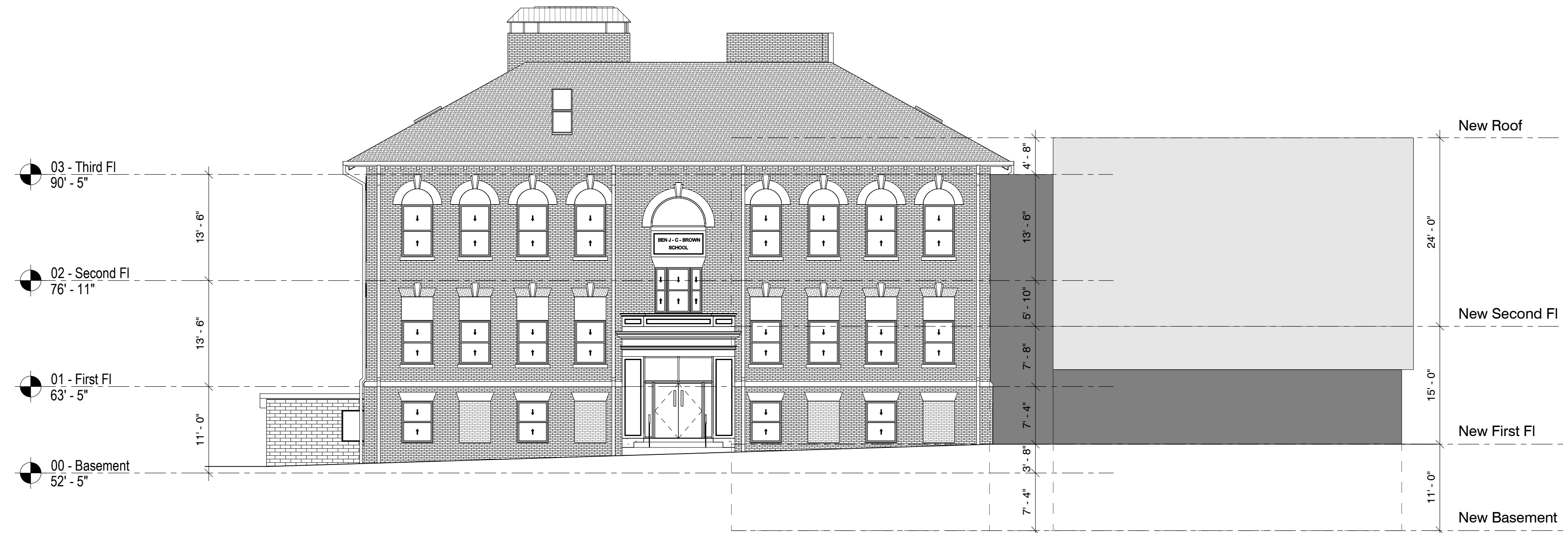
1 Proposed West Elevation - with Addition Massing A-5 3/32" = 1'-0"
