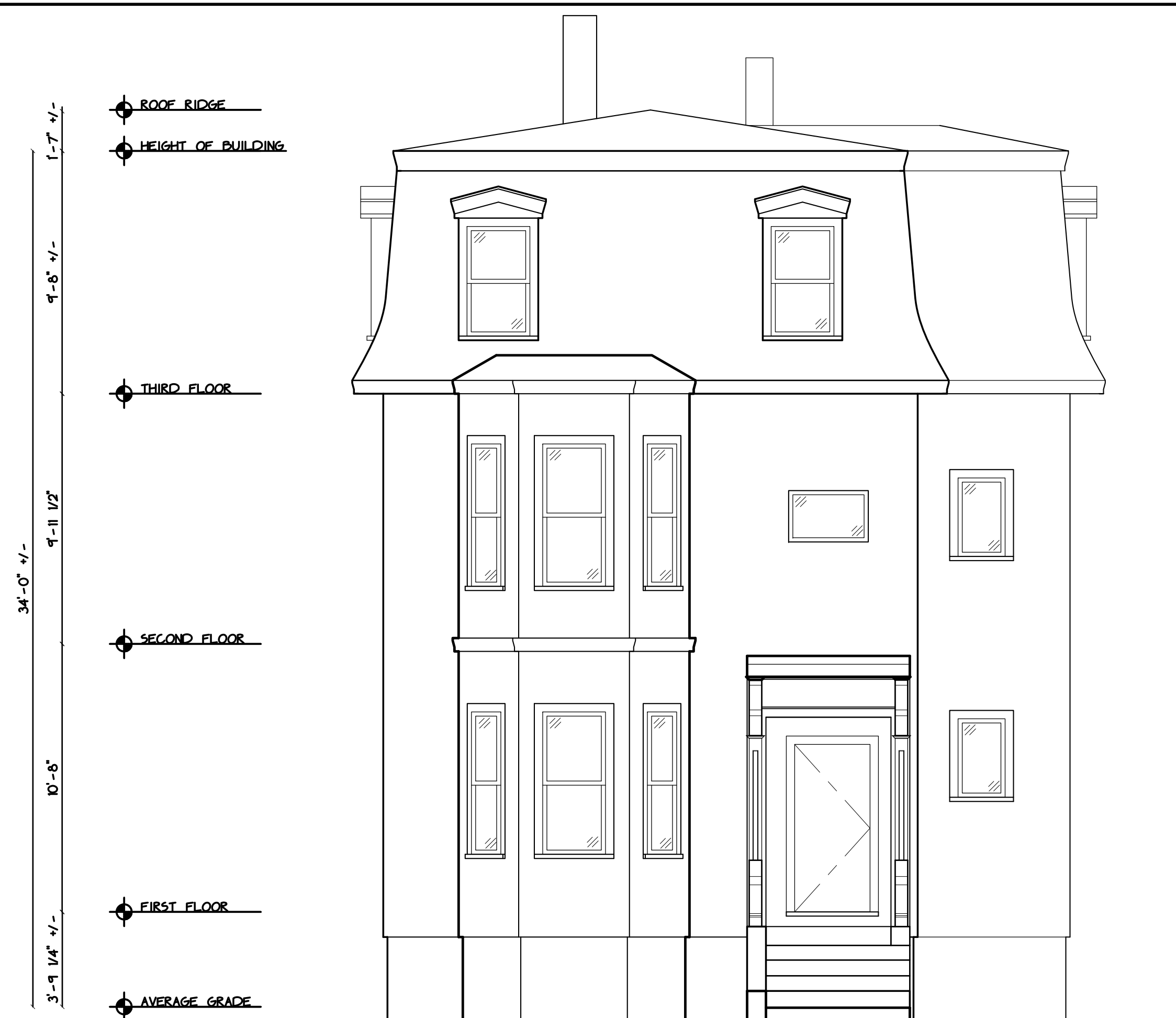
① Existing North Elevation Scale: 1/4" = 1'-0"
