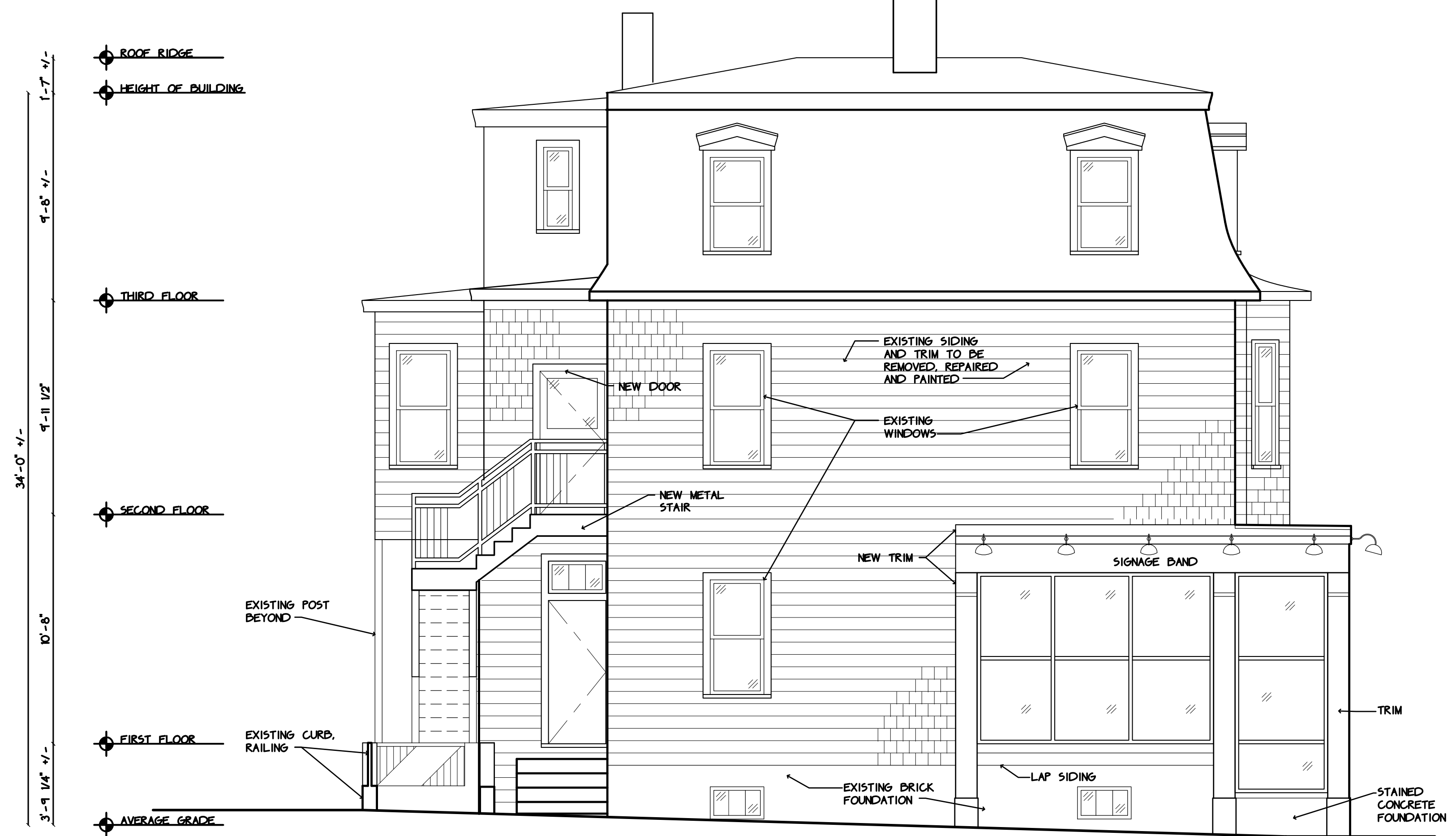
③ Proposed East Elevation Scale: 1/4" = 1'-0"
