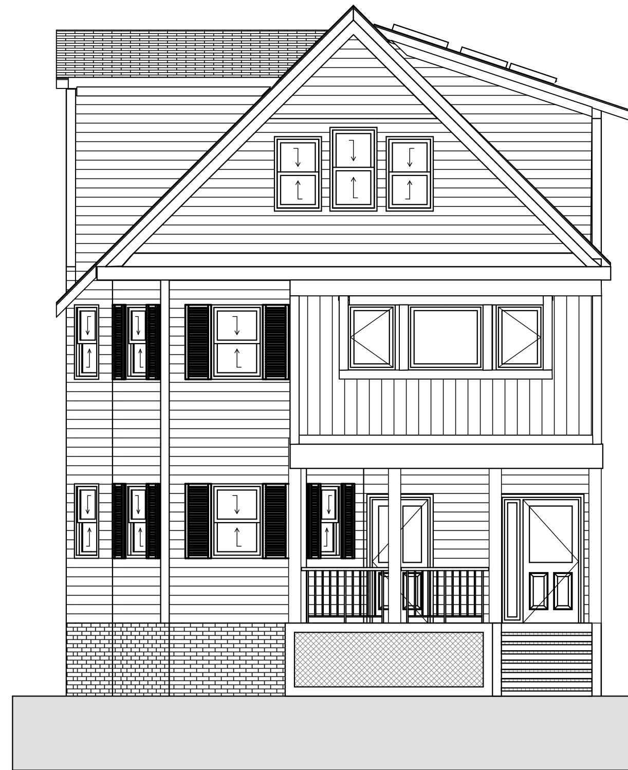
2 EAST (STREET) ELEVATION - PROPOSED SCALE: 3/16" = 1'-0"
