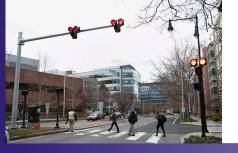
"HAWK" stands for High-intensity Activated crossWalK, which is a new type of traffic signal found in Somerville and the greater Boston region. It is intended to make crossing the street safer for pedestrians without forcing drivers to stop when there isn't anyone in the crosswalk. See the diagram below for instructions on how to use a HAWK signal as a driver and a pedestrian.
