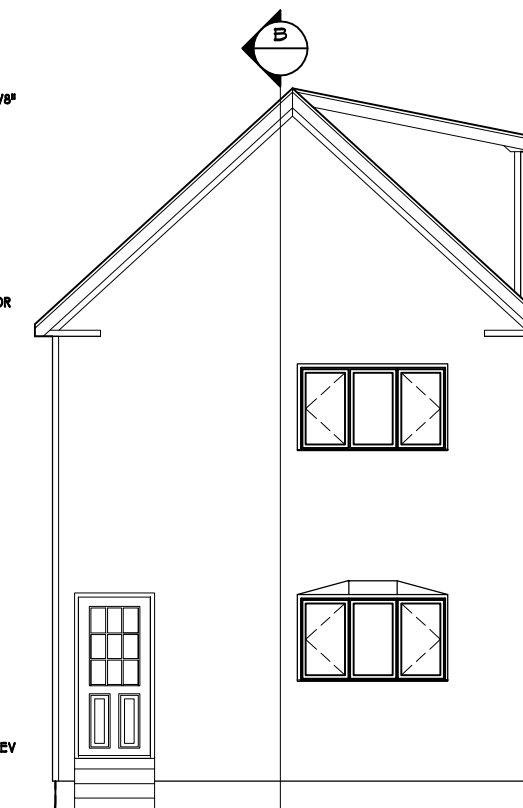
FRONT ELEVATION - EXISTING 1/8"=1'-0"
