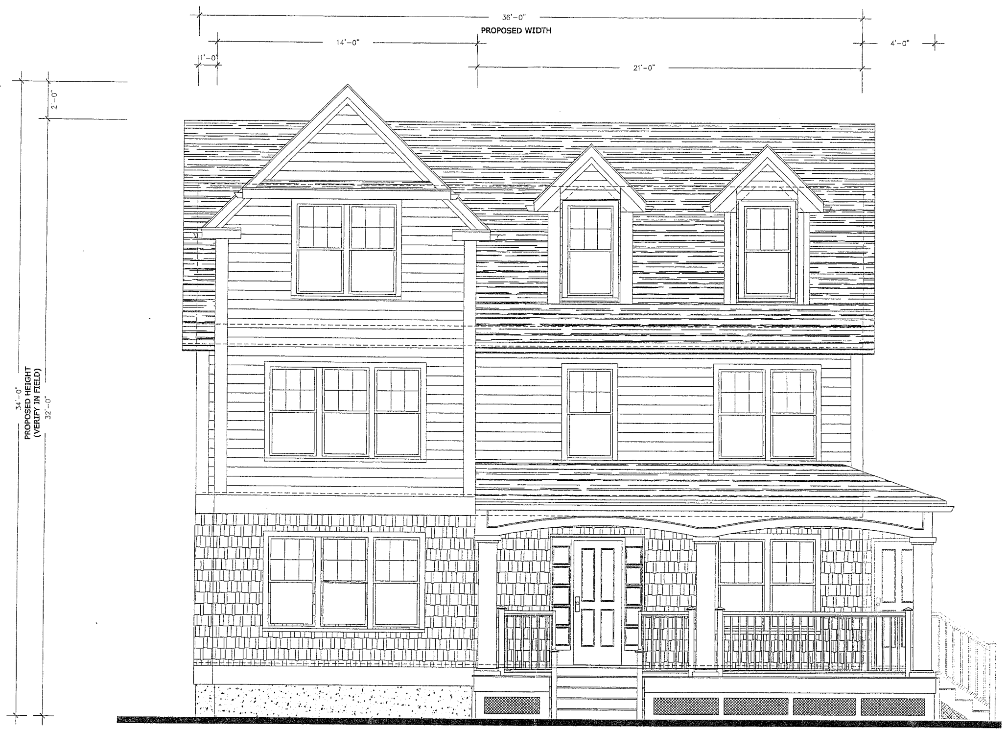
PROP. FRONT ELEVATION ESCALE 1"=1/2"
